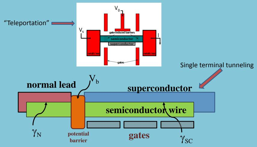
**Proposed Third set-up: Collect two sets of data**
