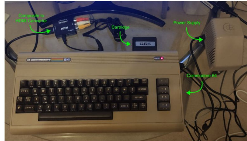
Figure 2: The experimental setup – a Commodore 64 is connected to a monitor through a composite video to HDMI converter, with the code cartridge inserted into the expansion port.
