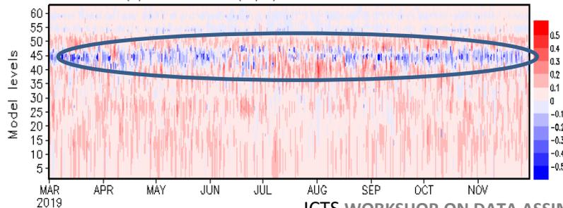
Differences in the monthly average of domain mean of analysis increment profiles for (a) Specific Humidity (mg/kg), (b) Potential Temperature (K), and (c) zonal wind (m/s). The model levels 15, 30, and 45 respectively represent approximate heights of 1.5 km, 6 km, and 14 km.
