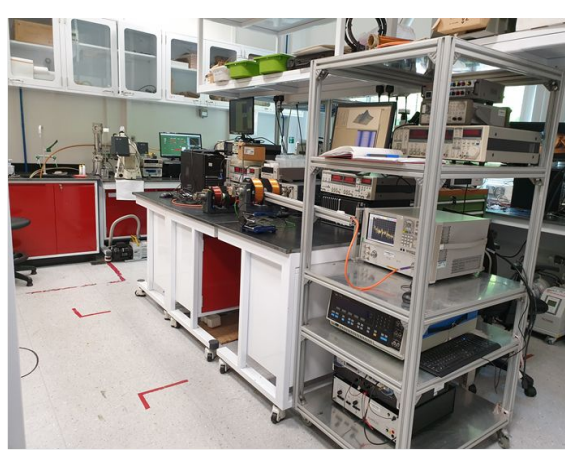
VNA based FMR spectrometer
