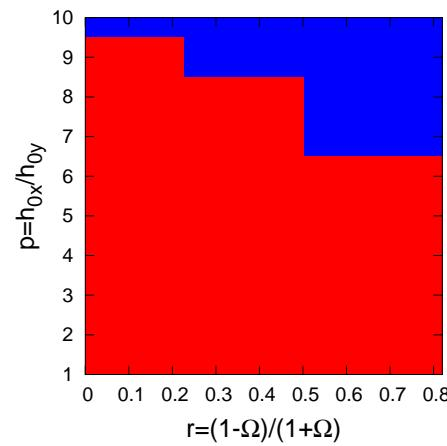
(a) The image plot of transition temperature (phase diagram) in  $p$ - $r$  plane. The transition temperature is obtained from the position of maximum of  $\text{Var}(Q_x)$ .
