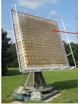
Closely spaced simple broad-band antennas No grating lobes: lower half of the band. ~400MHz to 1.4GHz. The FOV is ~200deg 2
