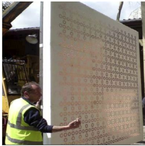
Closely spaced simple broad-band antennas No grating lobes: lower half of the band. ~400MHz to 1.4GHz. The FOV is ~200deg 2
