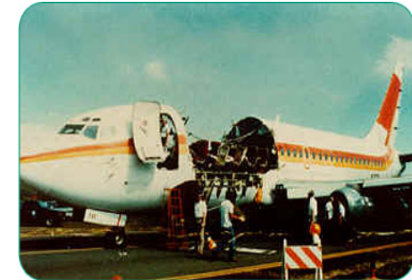
Aloha airline flight 243 fuselage failure (1988): Cyclic load, fatigue failure
