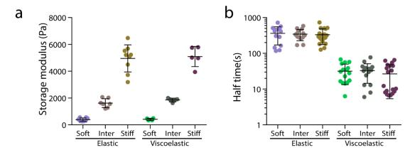
**Extended Data Figure 8. Quantification of hydrogel mechanical properties. a,** Quantification of the storage modulus of alginate hydrogels. n=8,4,5,7,9,5 gels per condition. **c,** Quantification of the timescale at which an initially applied stress is relaxed to half its original value. n=13,14,19,16,16,19 gels per condition.
